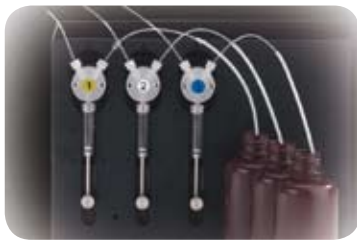
...up to three reagent injectors, programmable with individual injection volumes for each well
